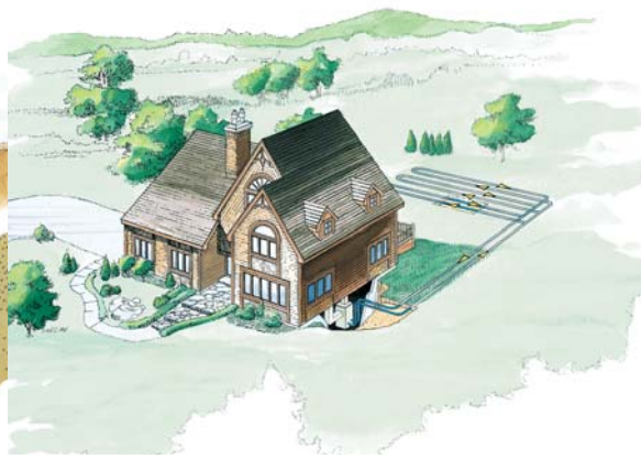
An example of a horizontal loop installation
